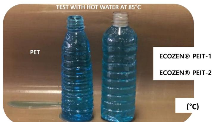
**Figure 2: PEIT grades exhibit much less shrinkage than PET when subjected to temperatures comparable to those associated with hot fill.**
