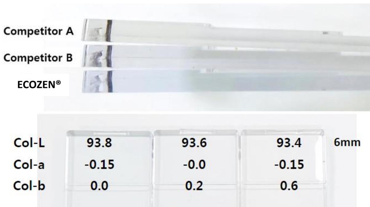
**Figure 3: PEIT grades containing low levels of isosorbide produce clear, transparent, almost colourless samples making them highly suitable for high quality cosmetic packaging.**
